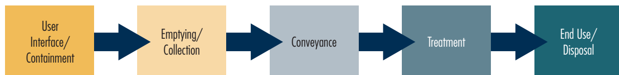
Figure 2.2 • The Sanitation Service Chain
