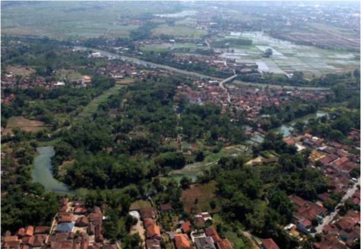
Citarum "Normalization" Program has changed the course of rivers when meanders are cutting off from the main stream, horseshoe-shaped OXBOW lakes are formed (above).
