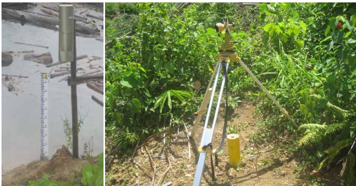
Figure 7. Monitoring on rainfall and water level (left); and land deformation (right)
