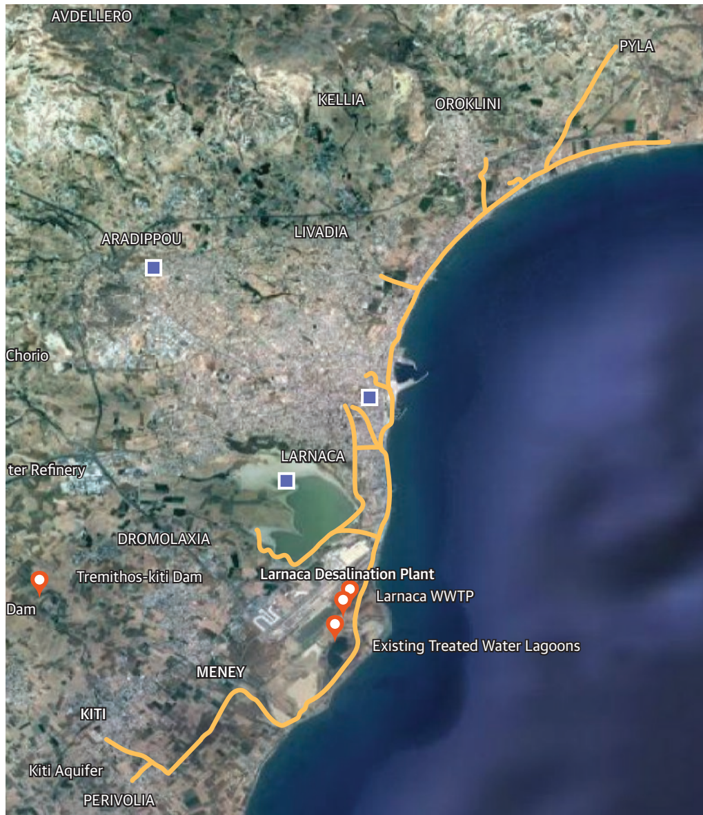
MAP 2.6. Treated Wastewater Conveyance Network in Larnaca
