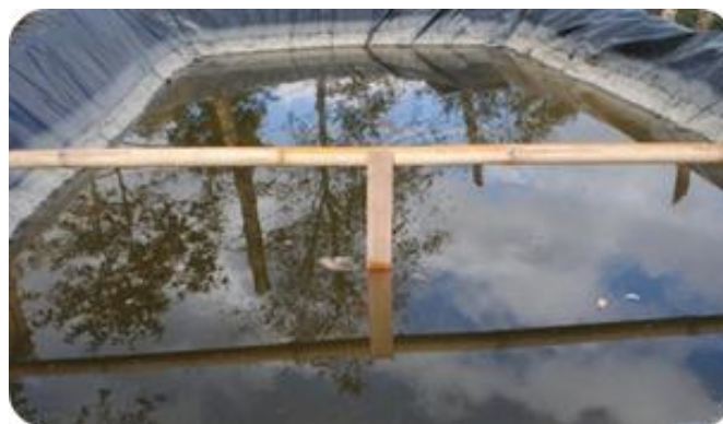
Figure 10. Stage provided for measuring the depth of stored water.
